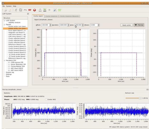
to a vector sum of 300 kV. Figure 2 shows the global vector sum GUI screen shot at 10 kW.
