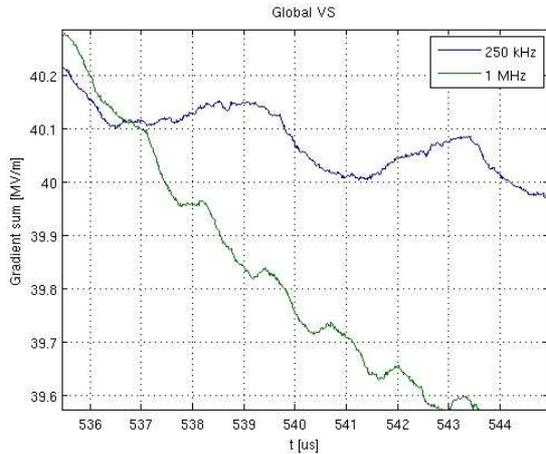
Figure 6: The vector sum beam transient zoom in shows individual bunch contributions for the two bunch repetition rates.
