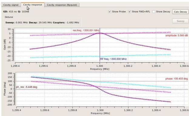
Figure 1: The response analysis of the EMMA cavity. The detuning, the loaded quality factor, the amplitude and phase response and the cabling delays are available from the measurement.
