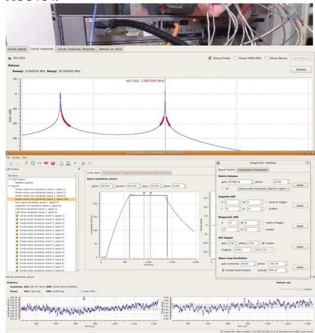
Afterwards beam transients measurements were carried out. The ACC456 vector sum flat top was loaded with 30 1.2 nC bunches at the repetition rates of 250 kHz and 1 MHz. From the acquired beam induced transients individual bunch contributions were clearly visible.
