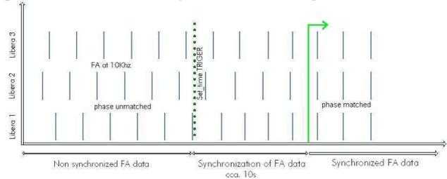
Figure 2: The FA data synchronization process.
