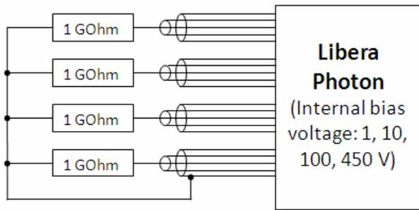
Figure 1: The measurement setup at lower ranges.
