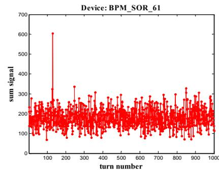
Figure 2: First beam at PETRA III. Response of a single BPM near injection. Due to an adjusted timing offset the first turn appears in turn no. 129.
