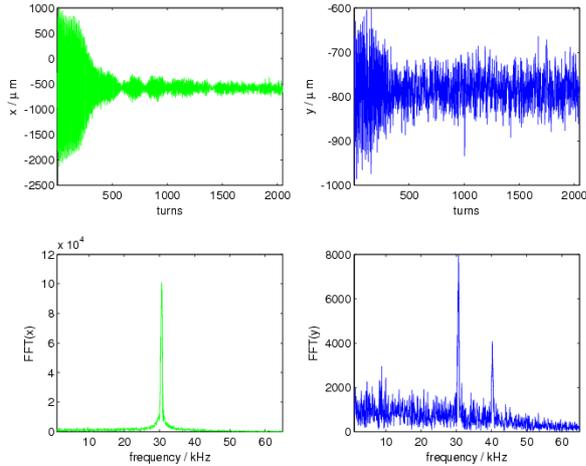
Figure 4: Horizontal and vertical turn by turn data together with FFT for tune measurement.
