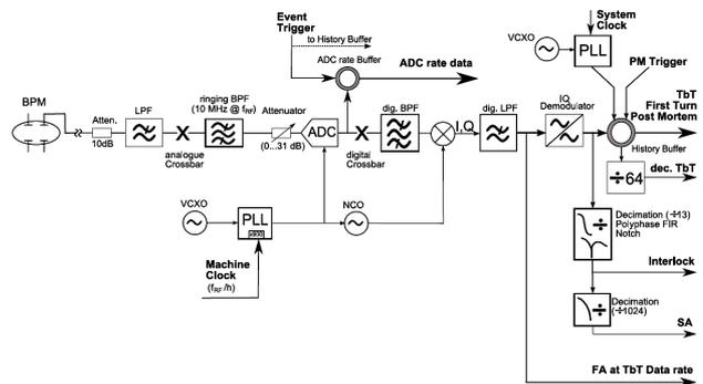
Figure 1: Functional block diagram of one channel of the Libera Brilliance BPM read-out electronics at PETRA III.
