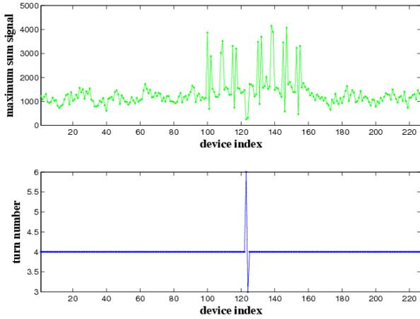
Figure 3: First turn sum signals from 227 BPMs observed at the same turn. Top: un-normalized sum signal. The narrow gap BPMs near the undulators are clearly visible. Bottom: Due to a readjusted delay the first turn appears in turn no. 4 now. BPM no. 121 and 122 are not installed.
