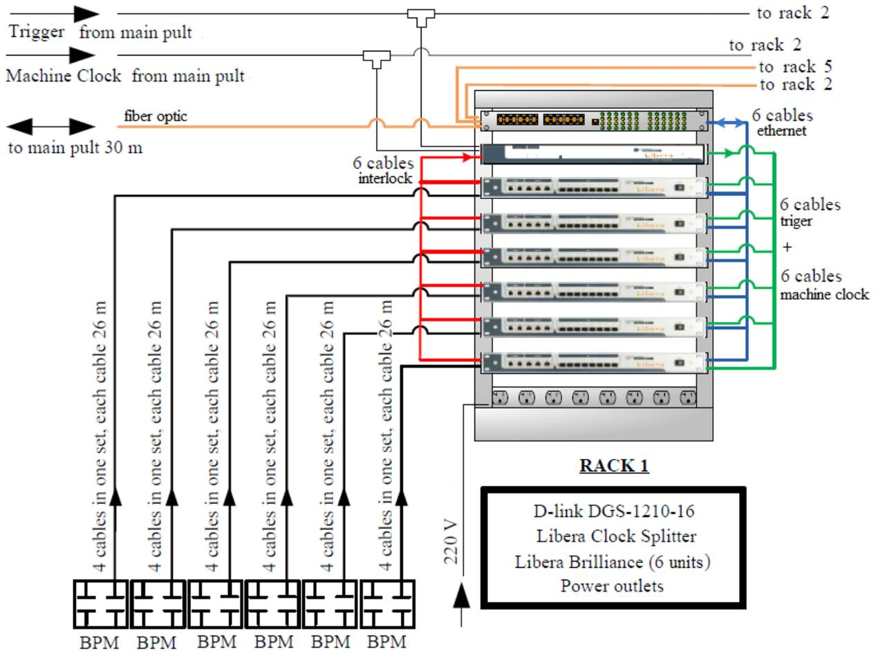
Figure 2: One rack with electron beam reference orbit measurement system equipment inside and all connections general layout.
