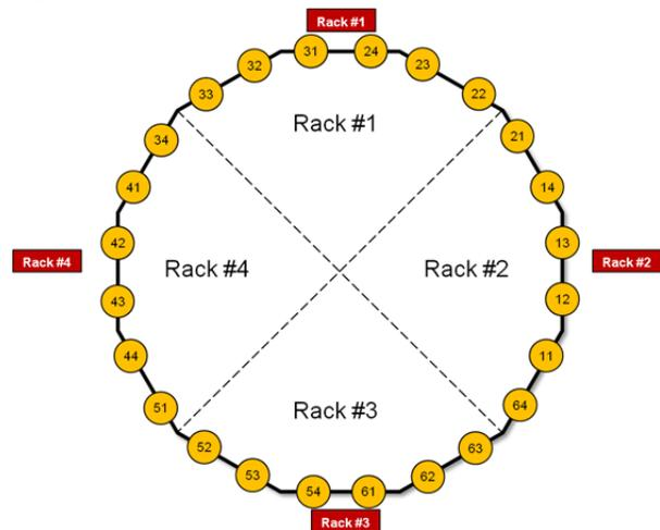
Figure 1: Distribution of BPMs and electronics.
