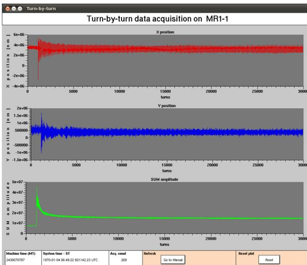
Figure 5: First turns on the BPM after injection point.
