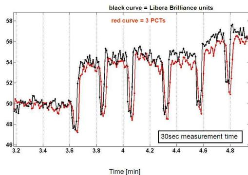
Figure 10: The zoom into real beam lifetime measurements.
