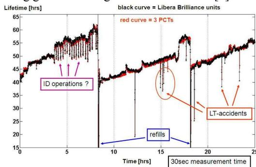
Figure 9: The measurements from both systems match and reveal the same phenomena.
