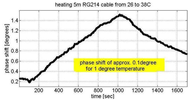
Figure 6: The curve shows a phase drift of 1.3° for a 12°C temperature variation.
