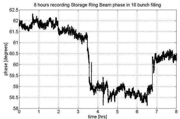
Figure 7: Recordings of the storage ring phase evolution over an 8 hour period (16-bunch filling mode).
