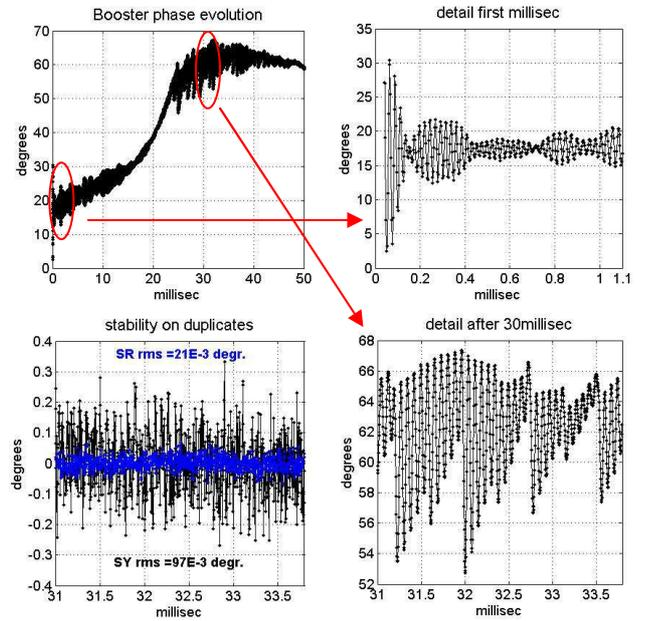
Figure 3: Phase evolution and phase oscillations of the booster beam during its 50ms acceleration cycle.
