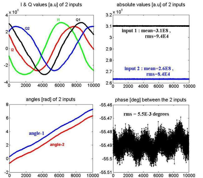
Figure 1: The I/Q values of two identical RF signals in a single Libera unit (upper-left) and the final differential phase values (lower-right), over a  $\sim 2$ s recording at 5.5kHz.
