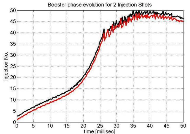
Figure 4b: SY phase evolution during the acceleration cycle between the first (black) and the last (red) injection of a refill.
