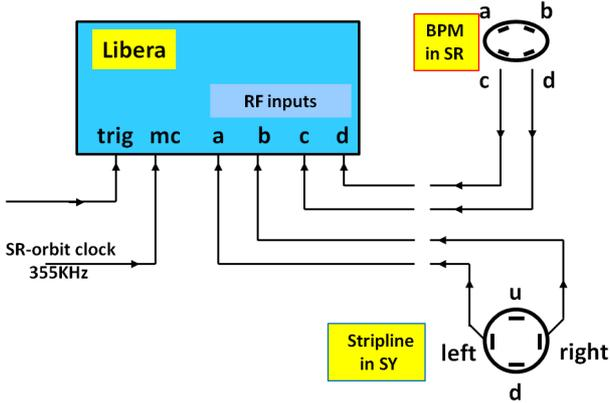
Figure 2: The hardware and interconnections of the phase measurement system between the storage ring (SR) and the booster synchrotron (SY).
