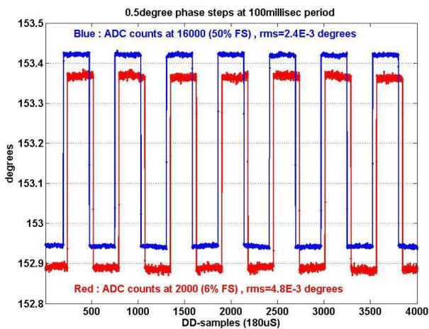
Figure 5: Recordings of phase modulation introduced by an electronic phase shifter.
