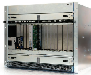
Figure 4: The MTCA.4. Crate. From left: Power supply, MCH, CPU, 2 x Libera Spectra module, space other 8 modules and/or another power supply.
