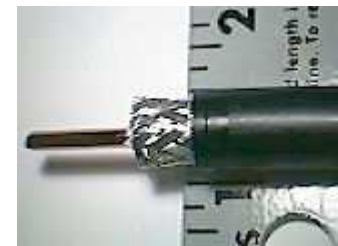
Major cable TIMES LMR400 Loss < 10dB/100m
