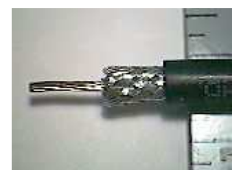
Jumper cable TIMES LMR240 Total loss < 0.5dB
