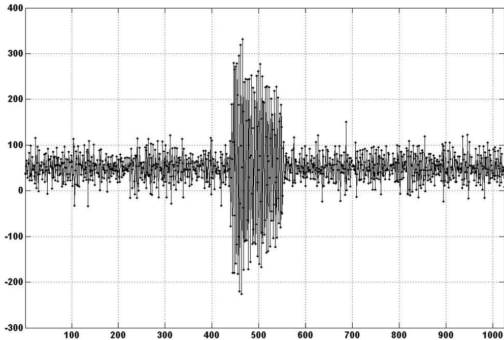
Figure 5: SUM of the ADC with 2 mA Injection from the Injector
