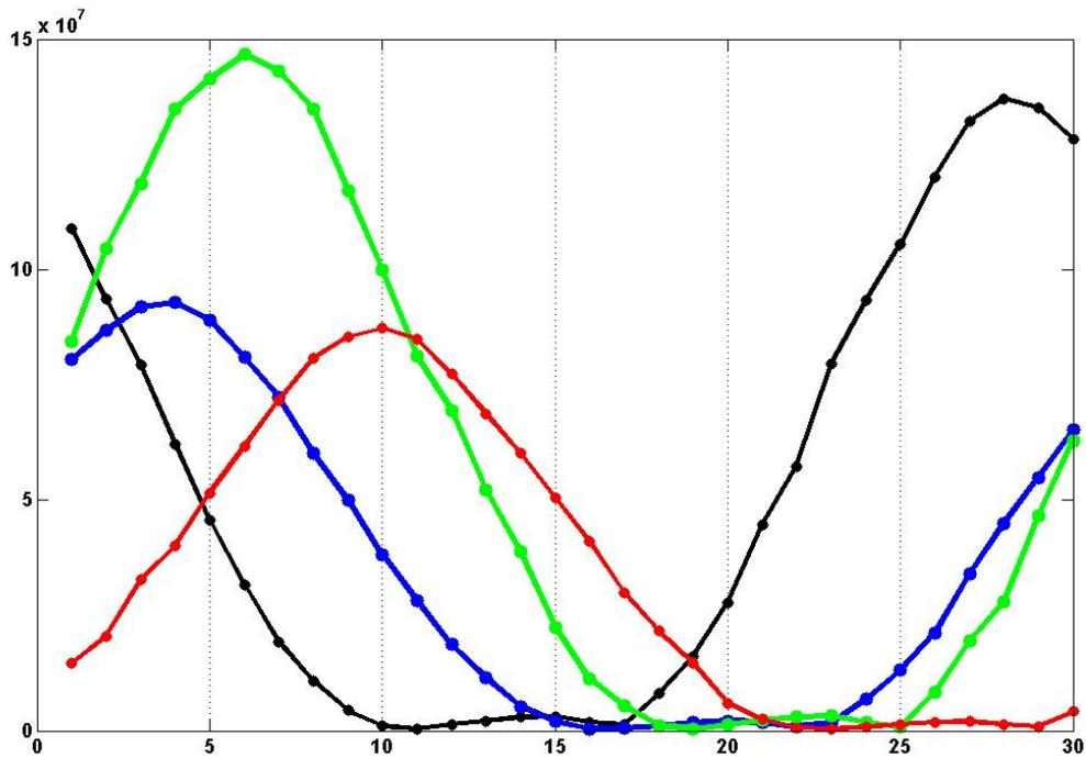
Figure 4: Scanning the 1/3 Summing Filter ('1 us long') Through the Full 2.8 us Storage Ring Revolution Period in 30 Discrete Steps of  $\sim 93$  ns.
