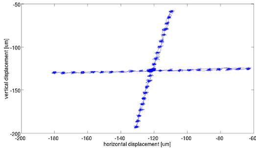
**Figure 4. Beam bump presented as XY plot.**
