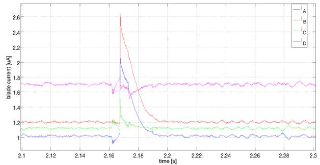
**Figure 10: Absolute current reading from each of the blades.**
