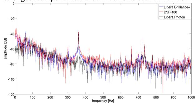
**Figure 5: Noise spectrum of three beam position monitors.**
