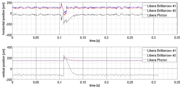
**Figure 9: Top-up injection as seen in the photon beam.**
