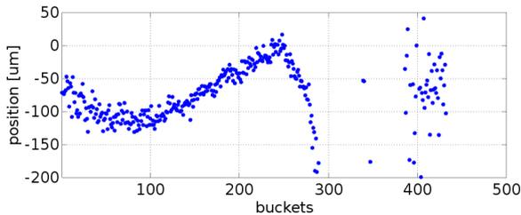
Figure 8: Position of every bunch within a turn. 10 mm scaling factor was used.
