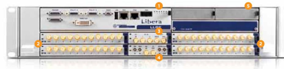
**1 Interconnection board (ICB):** implements functions of the QTCA Carrier Hub (MCH) with interfaces: 2x PCIe, 2x LXI, JTAG, RS-232, DVI, management USB, management ETH, USB and 2x ETH. A fast PCIe bus is used for the data transfer between COM Express module and AMC application boards. This high performance combination supports the implementation of low-latency control algorithms, real-time data processing and dedicated RF system diagnostics tools.
